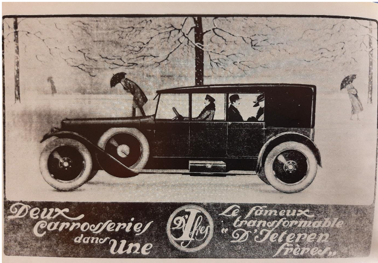
Picture 1 The famous Transformable D'Ieteren Frères made around 1923. The whole upper part of the car is retractable. It is the ancestor of our convertible cars.
